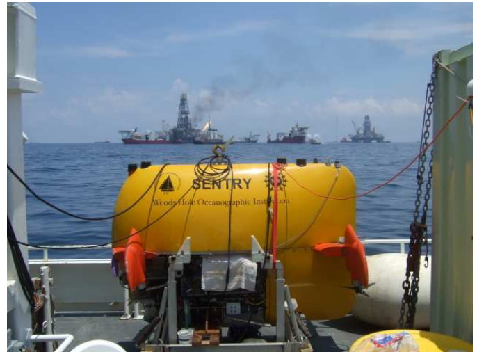
Fig. 1. The Woods Hole Oceanographic Institution AUV Sentry on the deck of the R/V Endeavor between deployments. Drilling platforms and other equipment working at the Deepwater Horizon blowout site are visible in the background. The closest to the site that the vehicle was deployed was 3 nautical miles (5 km). Photo by D. Yoerger.
