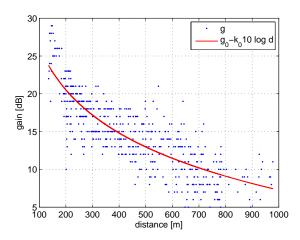
Fig. 1. Gain (normalized) vs. transmission distance. Dots show measured values; solid curve shows an estimated trend (a first-order logarithmic-scale polynomial fit to the ensemble mean at each distance yields  $k_0$ =1.9).
